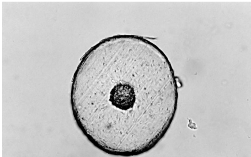
Figure 9 Photomicrograph of the bleached white human hair (Sample 7) treated with PEI ( M_n = 600 ) at 50°C and pH 7.9 for 60 min, then cross-sectioned and finally dyed with Orange II.
